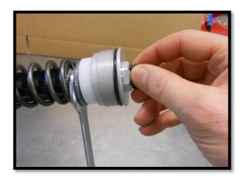
Unscrew the locknut to bring it in contact with the cap and tight with a 10Nm torque
