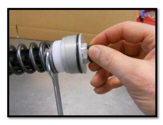
turn the adjuster knob clockwise to close it complete then open until it stop number the total click. They must be between 18 and 20. If more it means the front fork cap is not fixed correctly. In this case it's necessary to repeat the procedure from the start IMPORTANT: this control guarantee the correct assembling of this part
