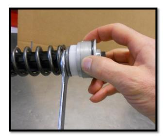
Screw in the front fork cap until it reaches the nut
