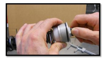
Holding the cap, screw in the adjusting knob 2 or 3 turns to engage the thread of the adjuster shaft
