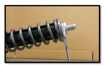
Preload the spring to free the space to insert the 19mm key
